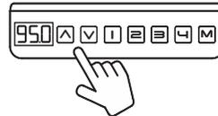
press ∨ for desired height adjustment
