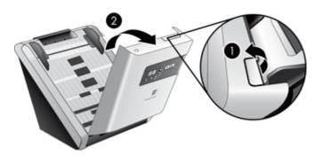
3. Open the roller cover on the inside of the scanner hatch and lift the roller up.
