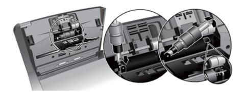
**6.** Open the door on the inside of the scanner, open the roller covers, and then remove the rollers.
