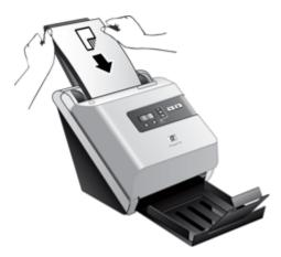
**6.** Verify that the paper guides are aligned with the edges of the stack.
