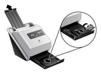
**2.** Adjust the paper guides to the width of the documents. Take care not to overtighten the guides, which can restrict paper feeding.
