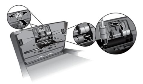
**4.** Remove any visible lint or dust from the roller and its housing using either compressed air or a clean lint-free cloth moistened with isopropyl alcohol.
